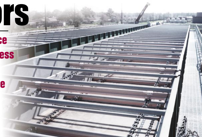
FIGURE 1. API separators have long been workhorse devices for refiners and petrochemicals manufacturers
