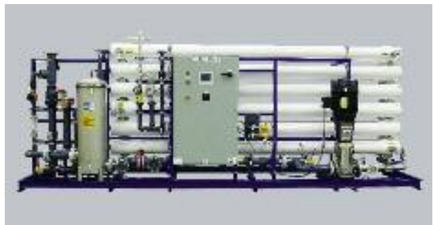
Reverse osmosis system
