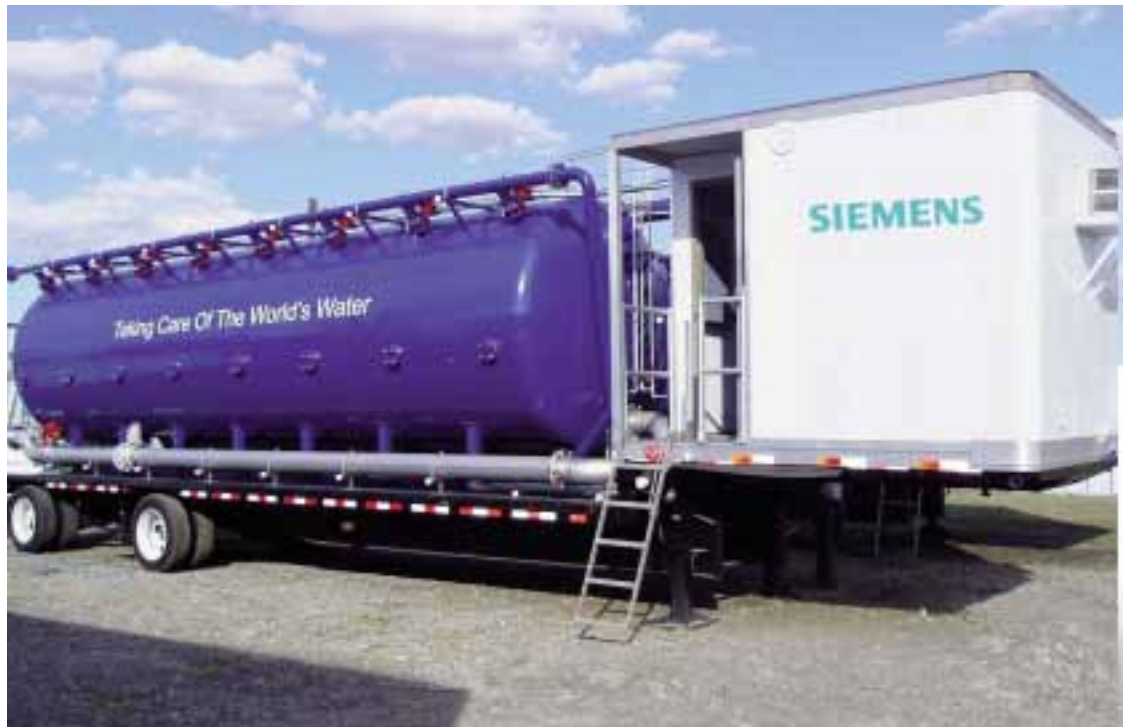
Mobile clarification and filtration system ensures uninterrupted drinking water supply without capital expense.
