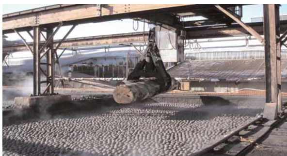
75% energy savings using E-Ball® floating tank cover.
