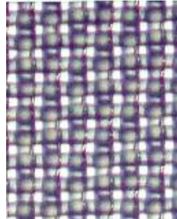
An absolute media rating is provided with woven media. (10-micron openings shown.)
