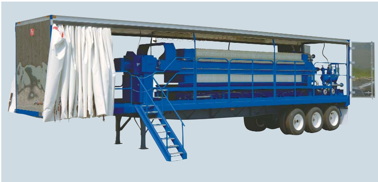
The Siemens mobile trailer system has a load capacity design of 80,000 lbs. The unit has four leveling legs, a rigid roof, stainless steel-clad, swing open doors and front bulkhead, and extra heavy duty weatherproof roller suspended side curtains for full access to both sides of the trailer. Six NEMA 4 lights mounted to the trailer roof provide ample lighting.
