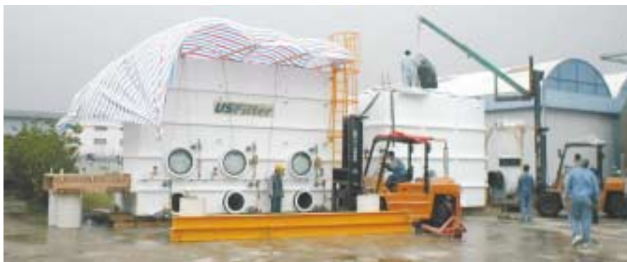
The LO/PRO® system handles air flow rates up to 65,000 ft 3 /min, treats multiple contaminants, has low operating costs and requires little maintenance.
