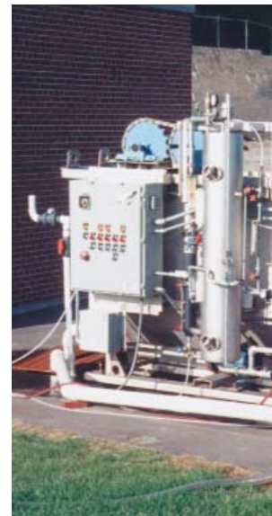
Folded Flow® separator pilot units are connected to existing plant lines and help establish design criteria.
