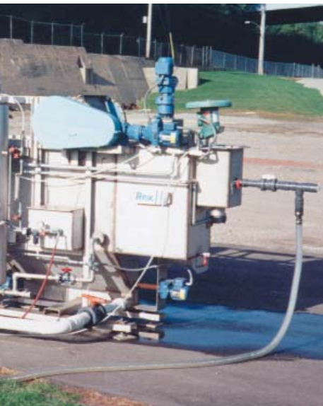
Units are available for test purposes. This test unit is easily moved and will quickly demonstrate the suitability of Floatation criteria for the full scale plant.
