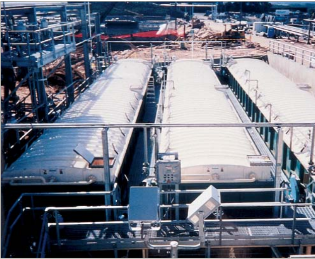
Figure 1. The API separator's heavy-duty design and ability to separate and continuously remove oily solids that can plug and foul other separation equipment has made it a preferred technology in heavy oil/ high solids applications.
