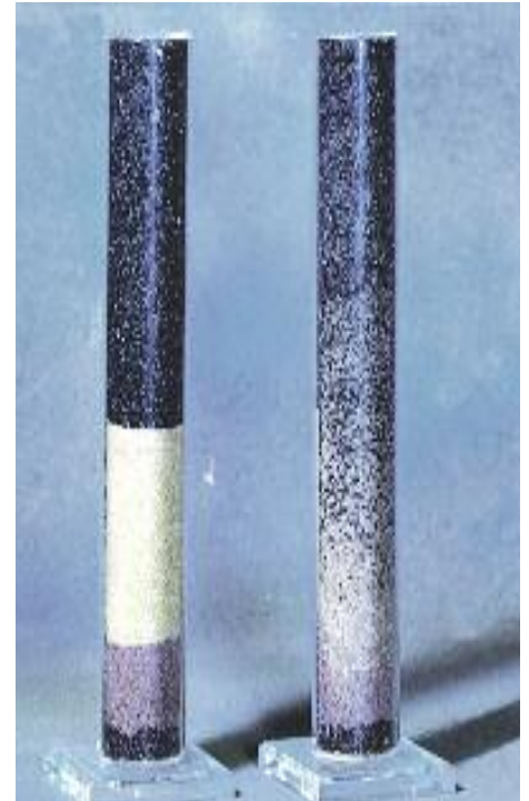
Mixed Media as placed (left) and after backwash.
