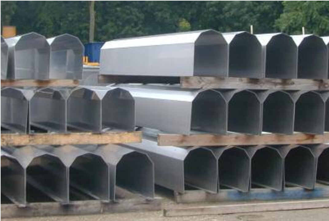
Launder system for rectangular clarifier.
