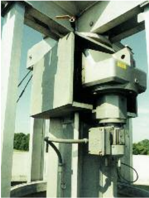
A MARD unit showing motor and enclosed drive.
