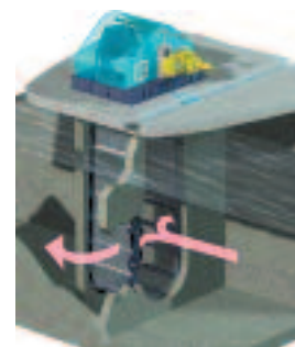
Center Flow Screens
