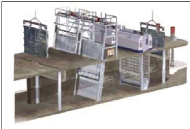
A typical cooling water intake structure arrangement.
