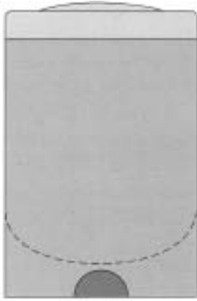
Tank Designed for Atmospheric Pressure (Must be vented)
