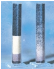
Mixed Media as placed (left) and after backwash.
