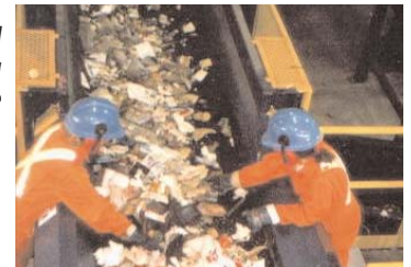
Front End Processor Picking Line
