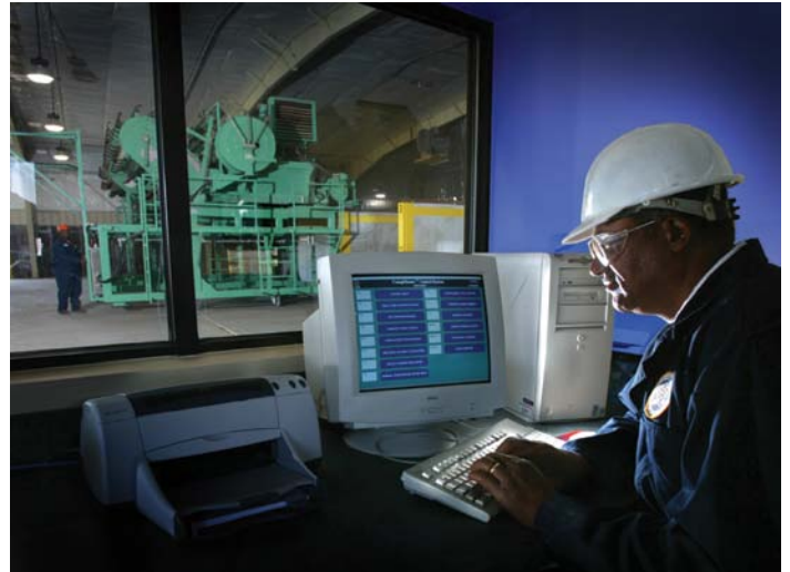
CompMaster® Control System Data collection, temperature regulation, aeration/moisture addition control, material/equipment tracking and report generation
