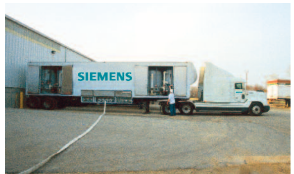
Mobile Demineralizers provide emergency response for the Cucamonga Valley Water District.
