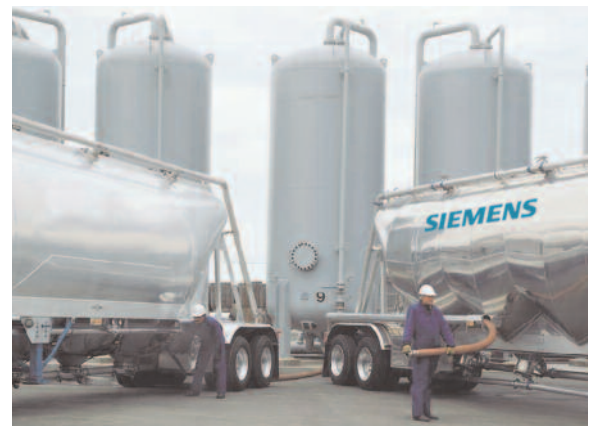
Manganese greensand was used to reduce iron and manganese at this construction site.
