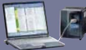
Commissioning of SED using PC software
