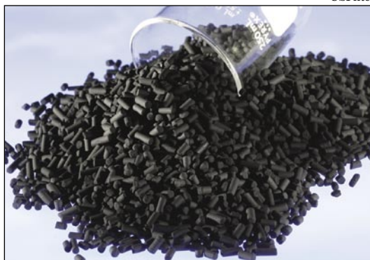
Though it looks much like any other activated carbon, Midas from USFilter has a powerful ability to oxidize H 2 S, thanks to the incorporation of magnesium oxide
